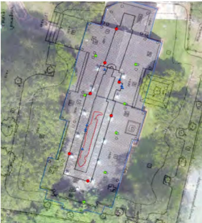
Figure 4: Layout and locations of IoT temperature and humidity measurement sensors
