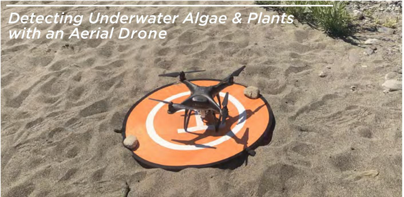
Figure 1: The unoccupied aerial vehicle (UAV) used for aerial image collection in this study.
